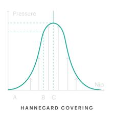
Furthermore, Hannecard combines specific properties of their covers with an optimized nip calculation. This allows the paper converter to obtain the required thickness, without having to press harder on the embossing roll.
